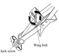
3. Turn the wing bolt completely to secure the jack.
